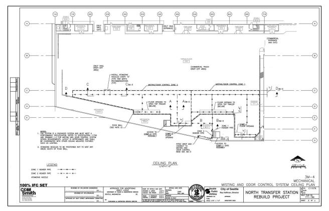
Figure 2-2: Spray Nozzle System Layout (From SPU Facility As-built drawings)
